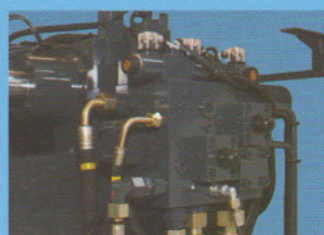
Manifold blocks closer to the actuator for faster response
